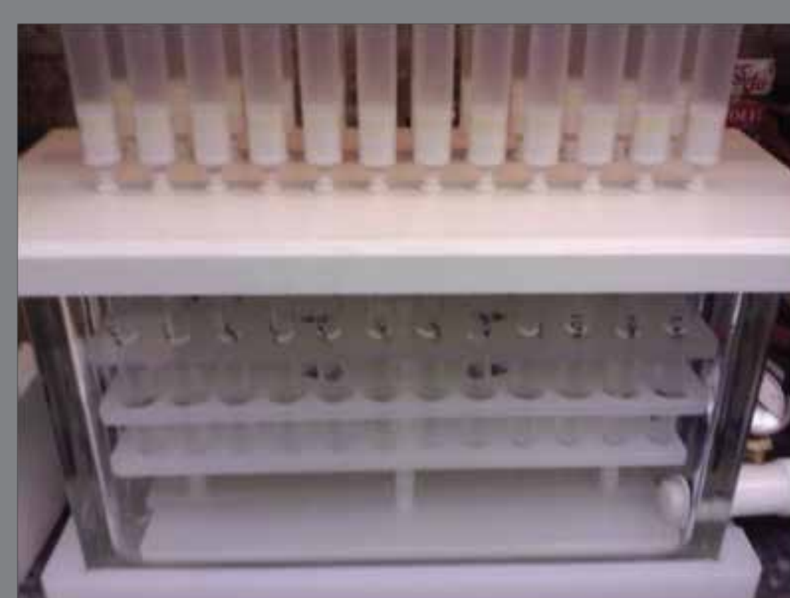
Cleanup of fish samples with dual layer SPE cartridges
