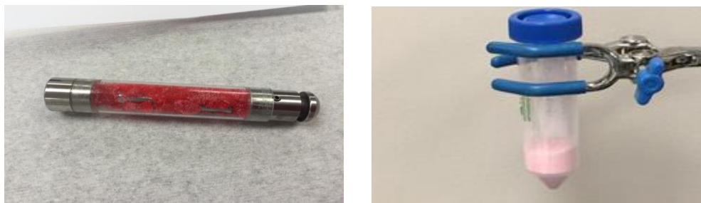
Figure 1: Hard candy before (left) and after (right) freezer mill grinding
