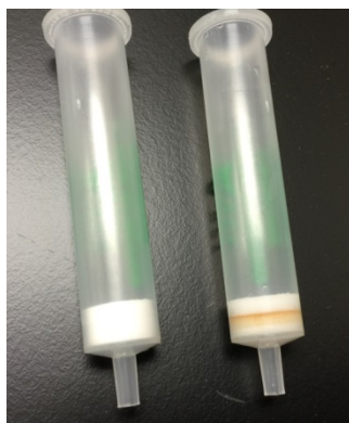
SPE cartridges: before (left) and after (right) horse urine extraction
